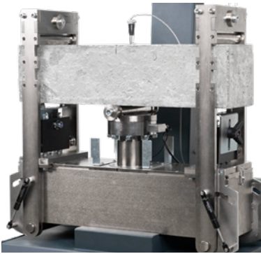
Deflection test on Steel Fiber Reinforced Concrete beams to EN 14651 [CMOD Method]
