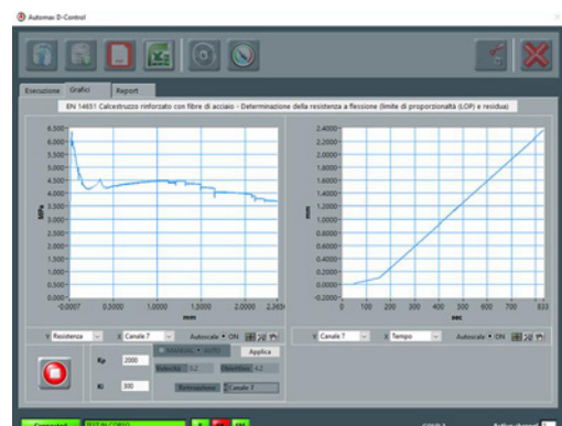
SW - Deflection test on Steel Fiber Reinforced Concrete beams to EN 14651 [CMOD Method]
