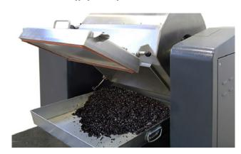
77-PV0077/C Detail of unloading. The mixing cylinder is rotated by a motorized tilting system for easy unloading. The tilting angle is adjustable to  $130^\circ$  to speed up the unloading operation
