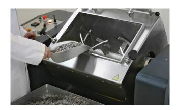
77-PV0077/C Detail of aggregate loading
