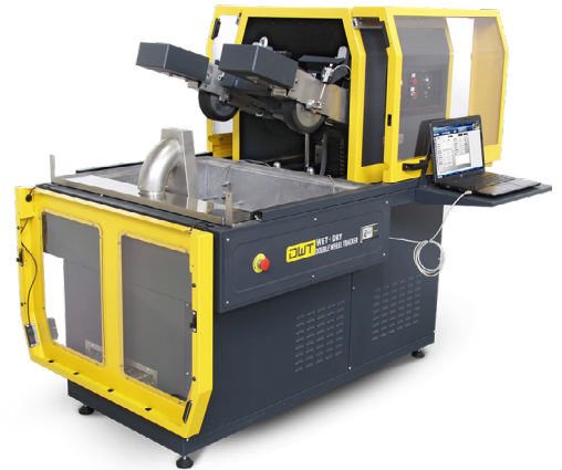
Detail of the motorized lifting system that raises the wheel assembly at the end of the test, making the use of hoists obsolete.
