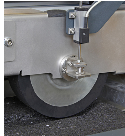
Detail of the motorized lifting system that raises the wheel assembly at the end of the test, making the use of hoists obsolete.
