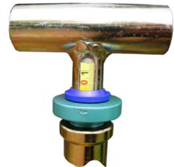
Standard set-up - showing adjustable zeroing nut (green), plastic cursor (blue) and clear scale (yellow)
